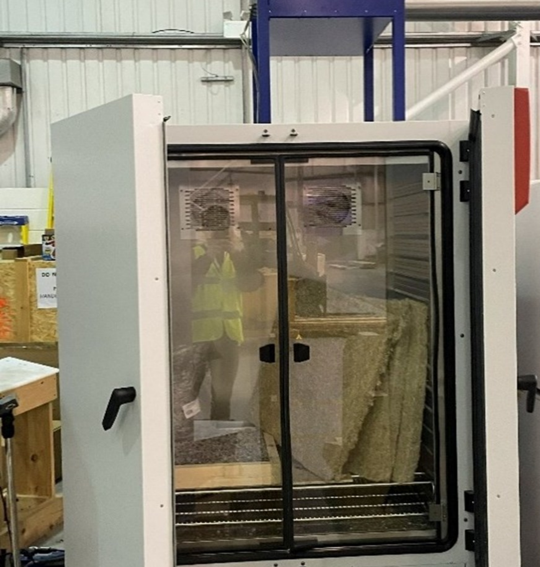
Climate chamber containing samples (left), insulation batts produced in factory and the surface images, acoustic test set up using impedance tubes (right)
